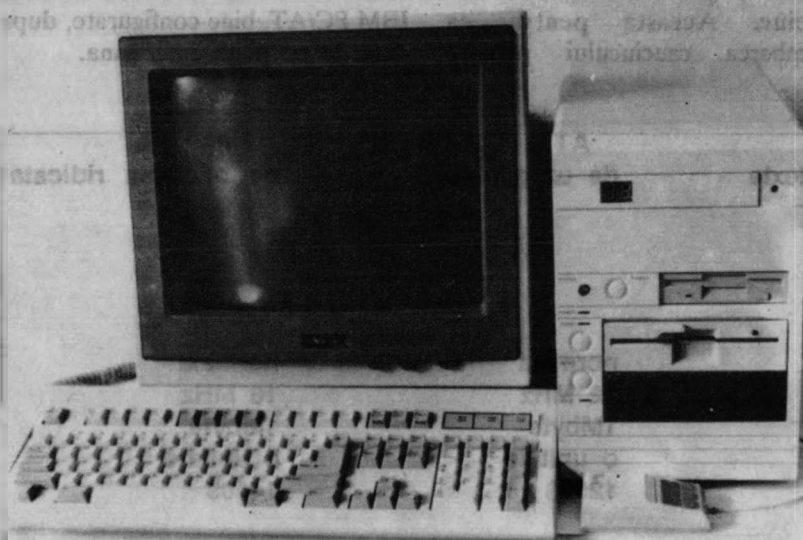
IBM-PC/AT 80386SX, 1 Mbyte RAM, 40 Mbyte HD, VGA
